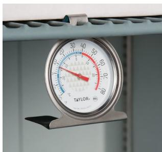
Thermometers are also required in every cold holding piece of equipment and hot holding piece of equipment. Cold holding equipment: shall have a thermometer in the warmest part of the cold holding unit, normally by the door.
